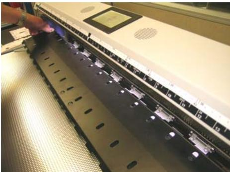
Picture 75: Moving the compensator plate upwards
