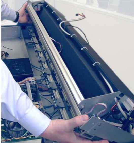
**Picture 66: Holding the glass plate rack**
