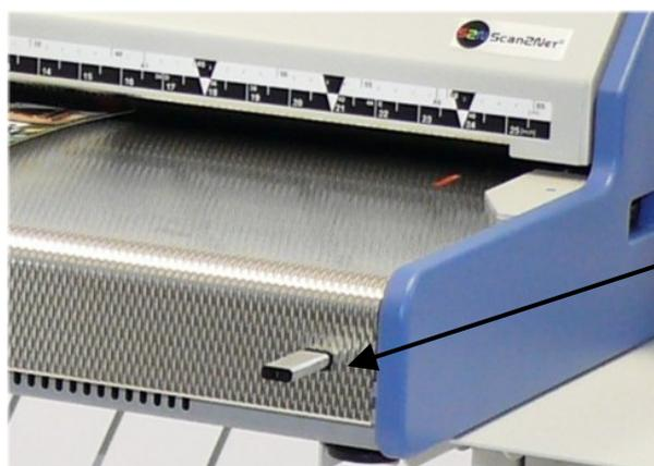
**Picture 85: USB stick inserted in USB connector**
