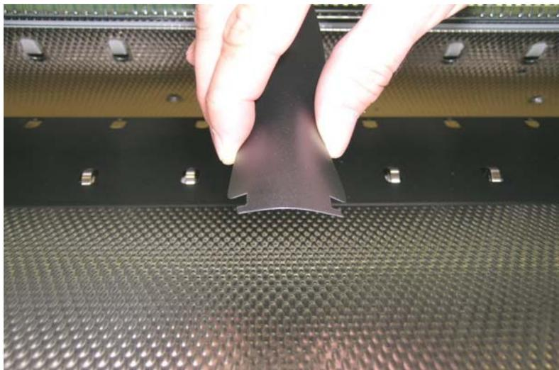
**Picture 6: Bending the paper transport wing**
