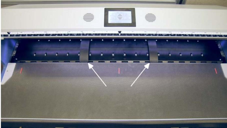
Picture 8: Position of paper transport wings
