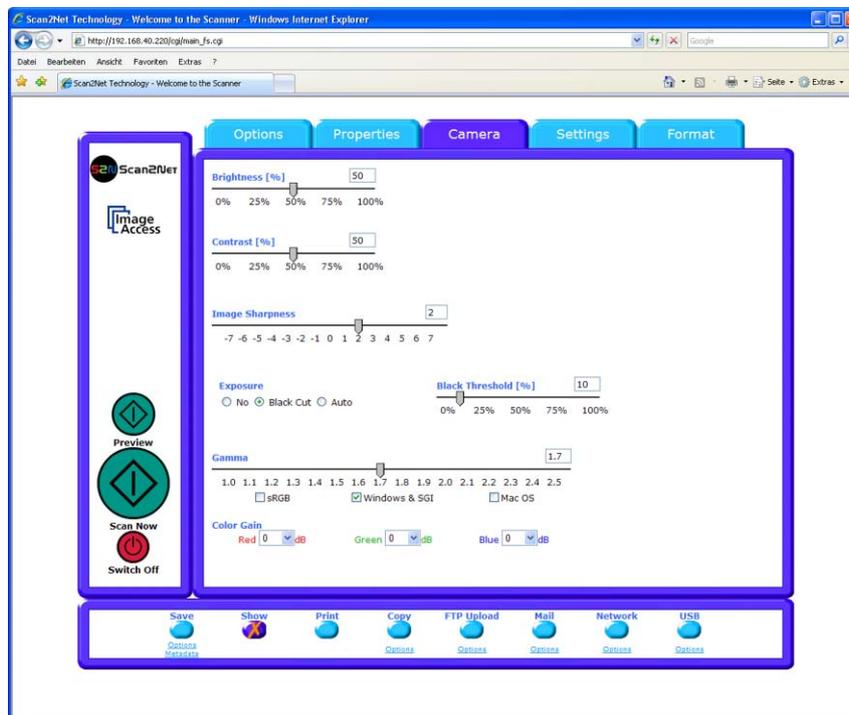
Picture 66: Exposure control slider
